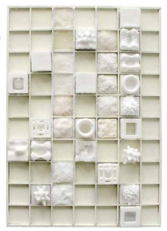
MATERIAL INVENTION BOARD- This board shows different Salt mixtures I tested to create a material which could be 3D-printed. The board shows Salt mixed with (i) Walgreens 92% rubbing alcohol- Ethanol (ii) Sake: Japanese rice wine (iii) Distilled Water
