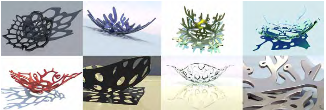
top: concrete cast, aluminum cast, thermo formed and laser cut tiles bottom: renderings of curved tiles experimenting with materials and colors
