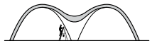
3. INVERT AND CONNECT Desiccate arches and invert. Grow arches together with new mat material.
