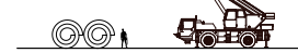
1. UNROLL MYCELIUM SHEETS Mycelium sheets consist of inoculated nutrients in two layers of quilted plastic composite. Sheets should be used within 24 hours of delivery.
