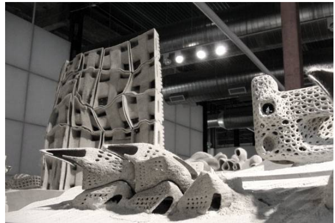
Figure 2. Earthscrapers exhibit demonstrating multi-part assembly systems for 3D Printing
