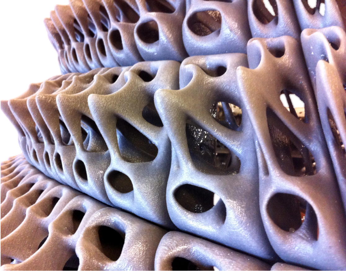
3D printed concrete polymer multiple-part assembly
