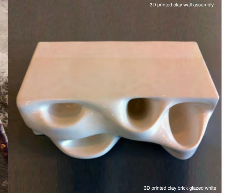
3D printed clay wall assembly
