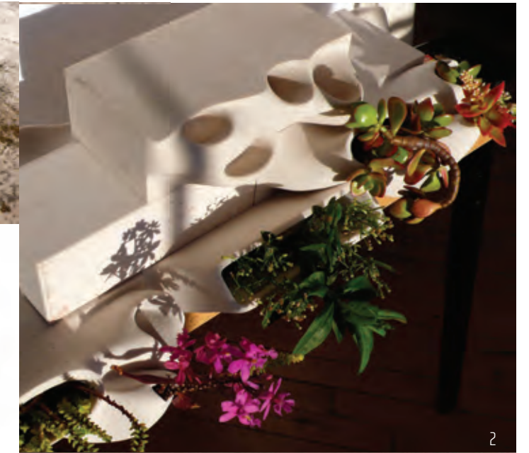
3D printed clay wall assembly
