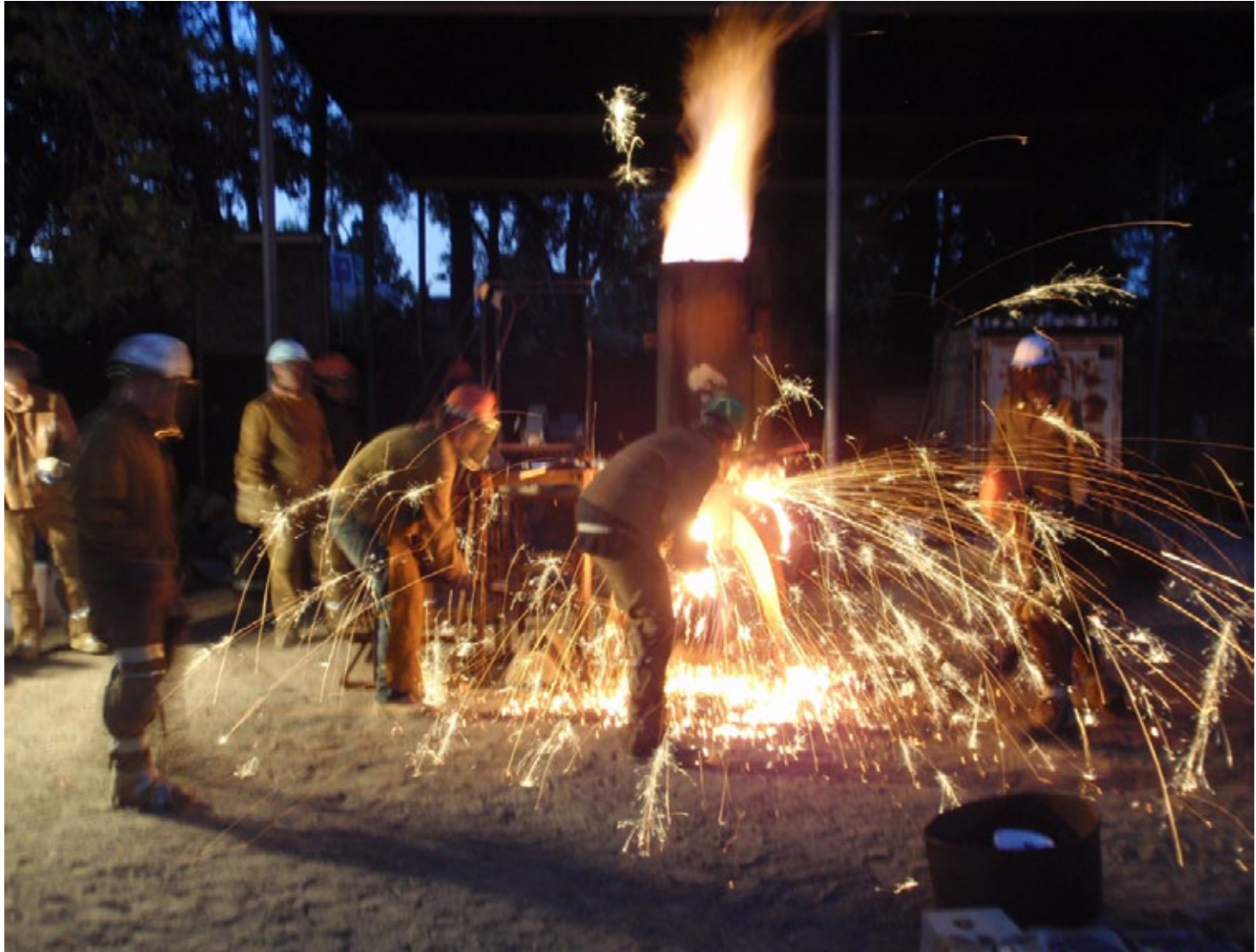
fig.0031 cupola iron casting, tapping the furnace ~ image credit george loisos.jpg
