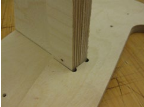
fig.0092 3.8125 router detail to avoid chiseling interior corners.jpg
