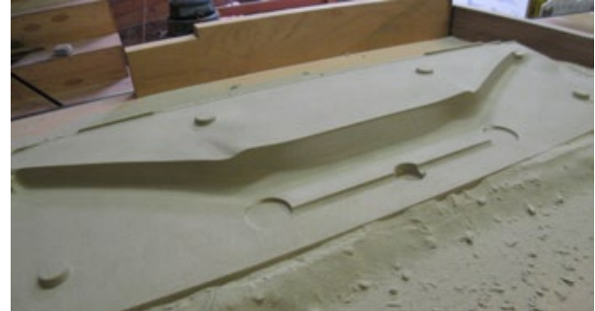
fig.0016 milled olivine sand mold for small floor member.JPG
