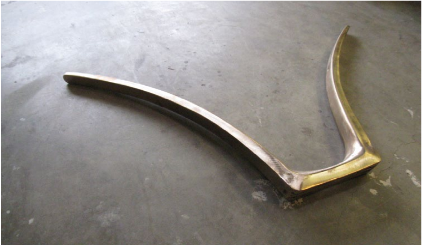
fig.0021 chased & completed casting ~ fl.3a.jpg
