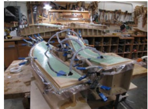
fig.0072 vacuum bagging composite parts.JPG
