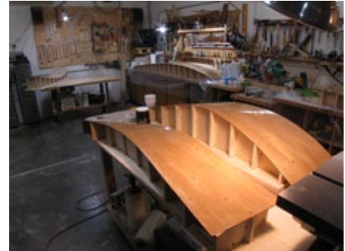
fig.0071 molds for fiberglass components.JPG
