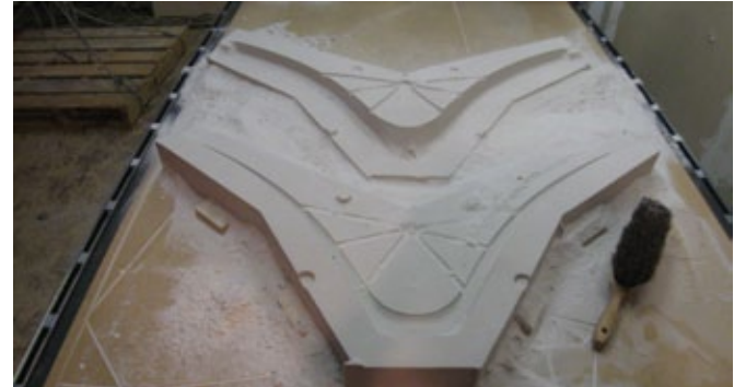
fig.0015 complete milled silica sand molds for a floor component.JPG
