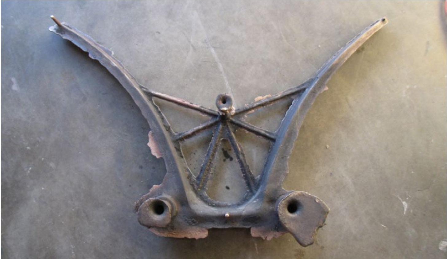
fig.0019 raw casting with gating &amp; risering ~ fl.3a .jpg
