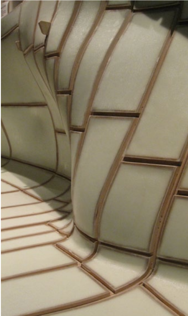
fig.0100 3.8125 glassed panels in place.jpg
