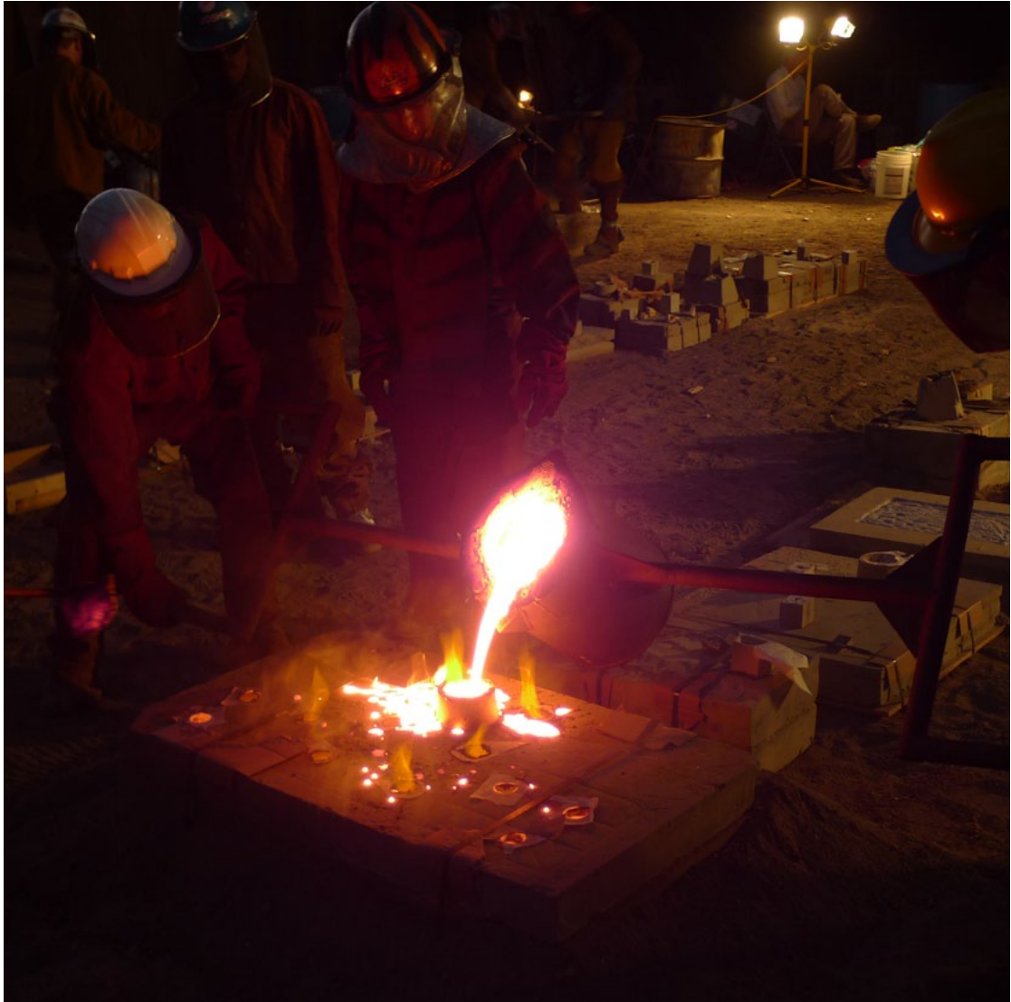
fig.0032 iron casting, pouring the small table – image credit nathan brown.jpg
