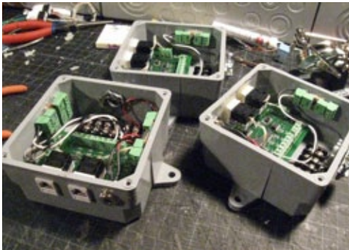
fig.0021g one-wire network digital & analog sensor hubs.jpg
