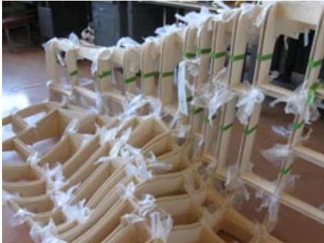
fig.0096 3.8125 gluing panel frames together in place.jpg
