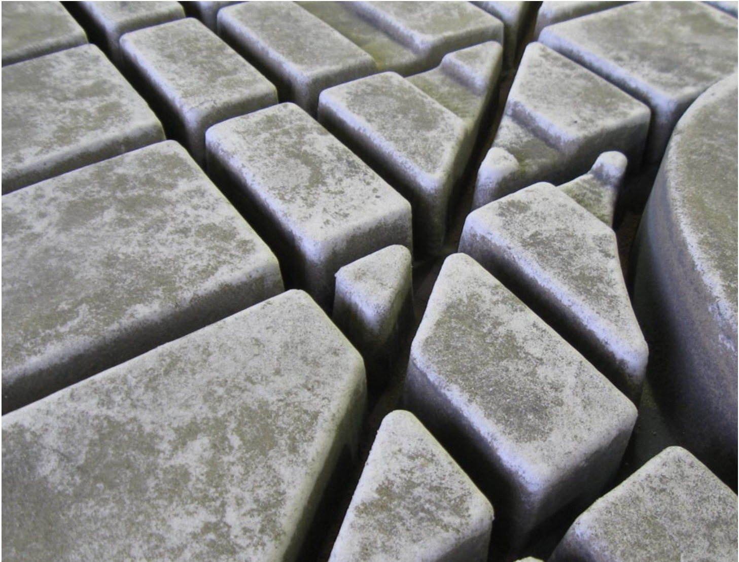
fig.0030 sand mold cavity detail ~ bandsaw table.jpg
