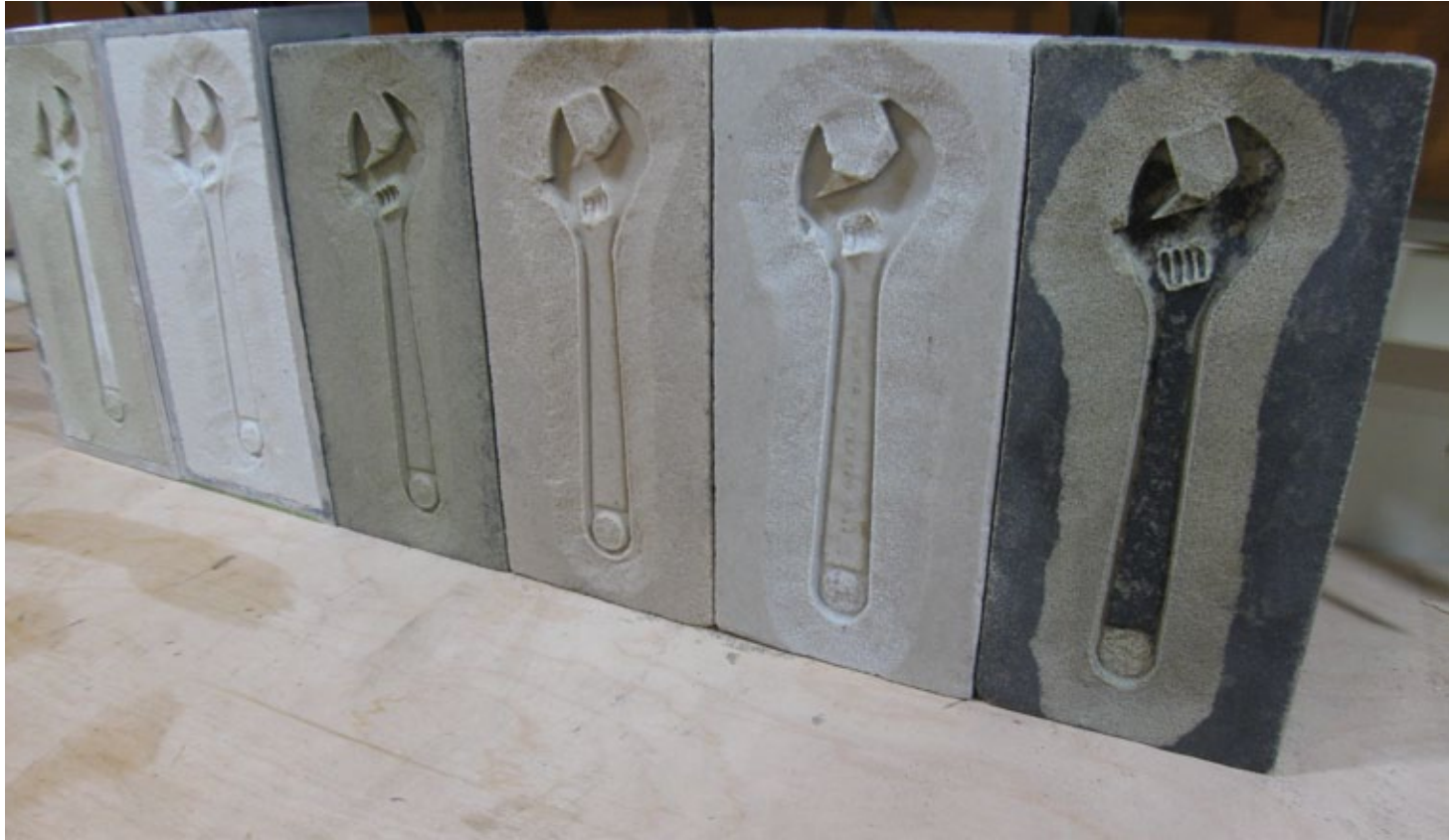
fig.0041 resin & sand density and resolution tests, with a wrench.JPG
