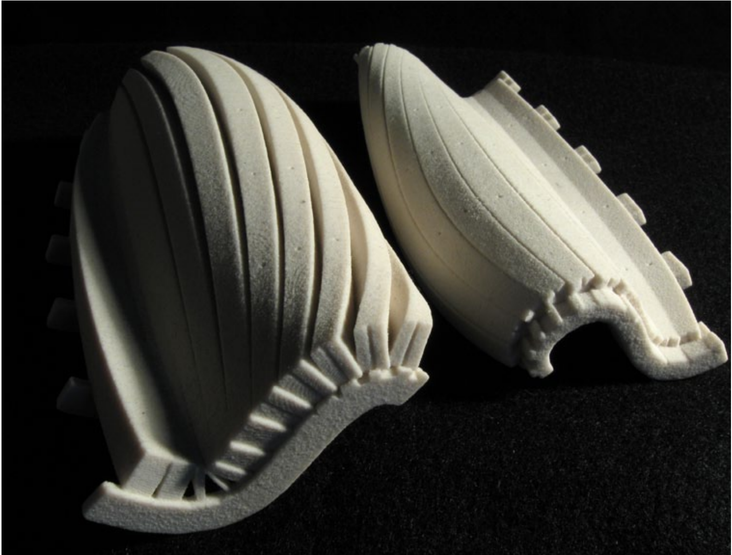
fig.0082 two different definitions of the same surface using different member sizes.jpg
