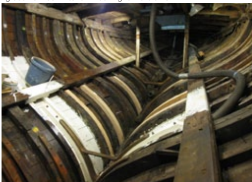
fig.0005 shireen interior ~ looking aft with new floor casting.JPG
