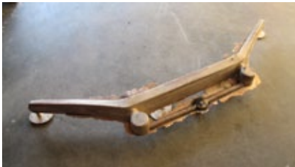
fig.0020 raw casting with gating and risering ~ fl.7a.jpg
