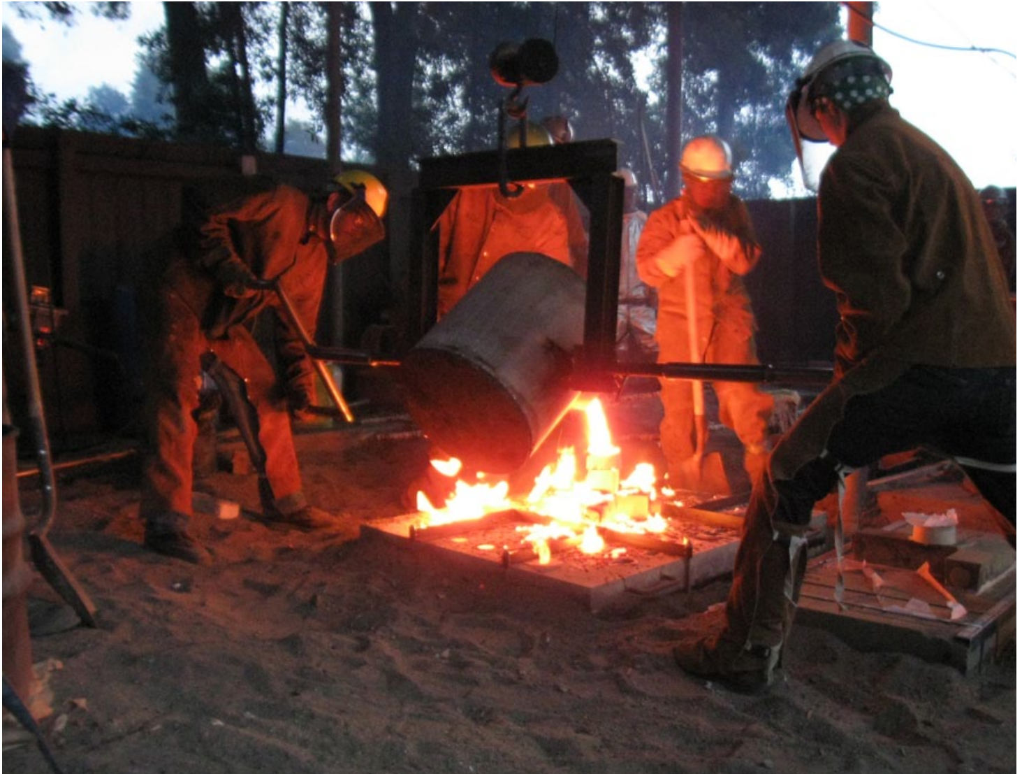
fig.0033 iron casting, pouring the big half with the bull ladle ~ image credit eleonor pries.jpg
